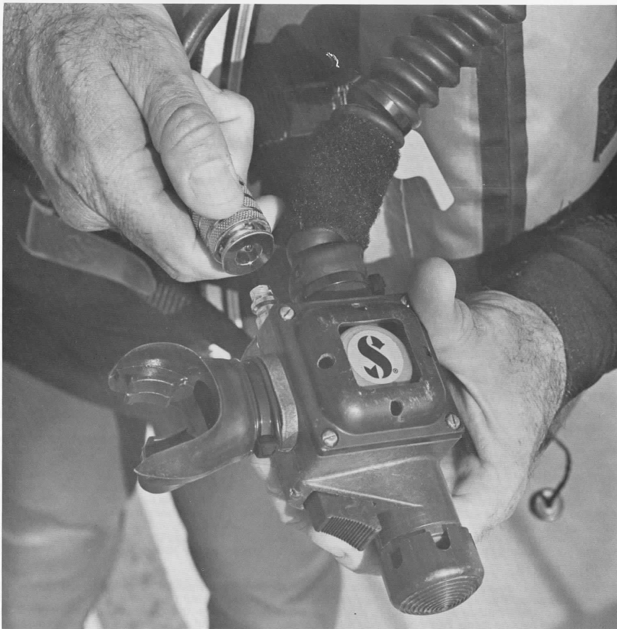
Attaching The Low Pressure Air Supply To The A.I.R. II
