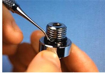
20) Remove the "o" ring from the Din Lockdown
