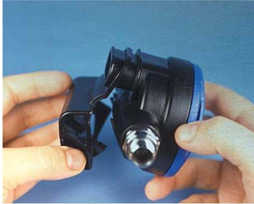
28) Install the mouthpiece and secure with a tie wrap
