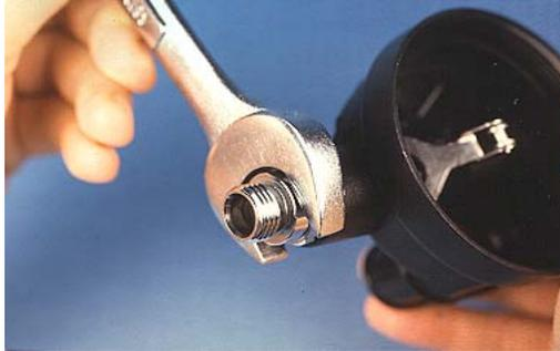
3) Using a 3/4 inch wrench loosen and the remove the Inlet Nipple
