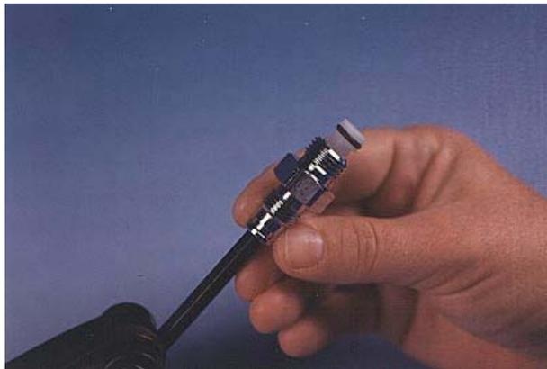
**After loosening the orifice completely use a 6mm Allen key to push the orifice
