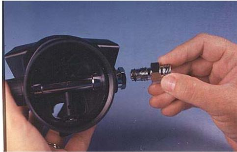
**Insert this assembly into the Adjustment tube**
