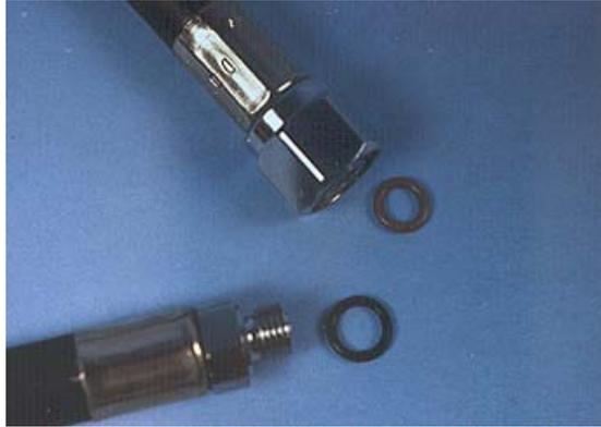
29) Lubricate and install “O” rings and on the low pressure hose. Install the hose into a LOW pressure port on the RG1200 First stage
