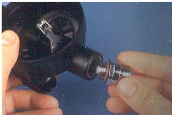
5) Temporarily install the Inlet Nipple
