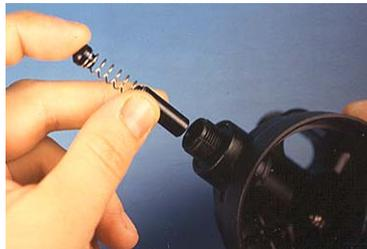
Clean and lubricate all the interior parts to the adjustment assembly
