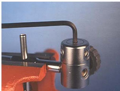
13) Insert a 6mm Hex wrench and remove the Turret retainer
