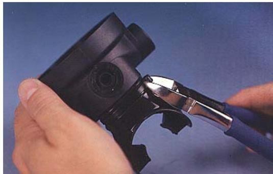
**Remove Mouthpiece RG1273 by cutting Nylon Tie**
