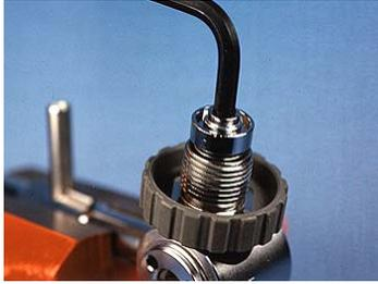
19) Insert a 6mm wrench into the Tank Inlet
