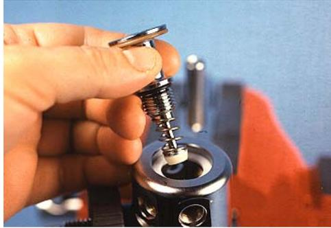
21) Tighten with a 6mm hex wrench ( Be careful not to crimp "O" ring )
