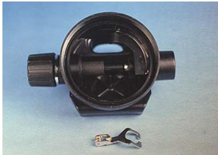
17) Remove the adjustment housing, remove the “O” ring from the housing
