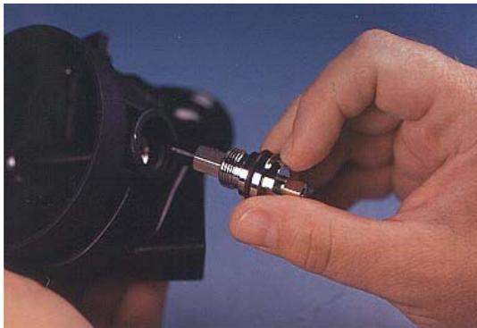
**The Adjustment Assembly can now be inserted into the Adjustment tube RG1405**
