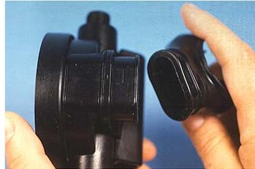
24) Use a small flat tipped screwdriver CAREFULLY pry the exhaust tee loose by using the small spaces provided under the Inlet and Adjustment tube ports
