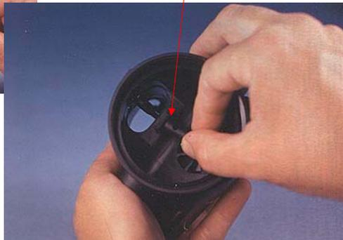
**The Deflect tube RG1422 can now be installed take note of the orientation. Small opening faces out
