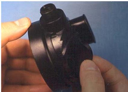
2) Install the Valve seat into the piston
