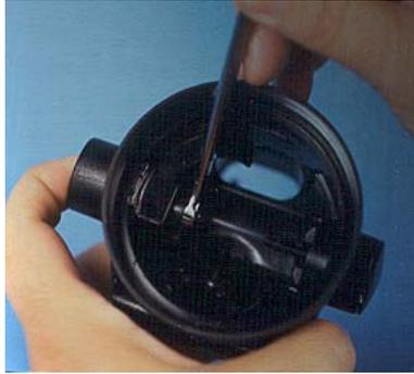
10) Remove the two spacing washers
