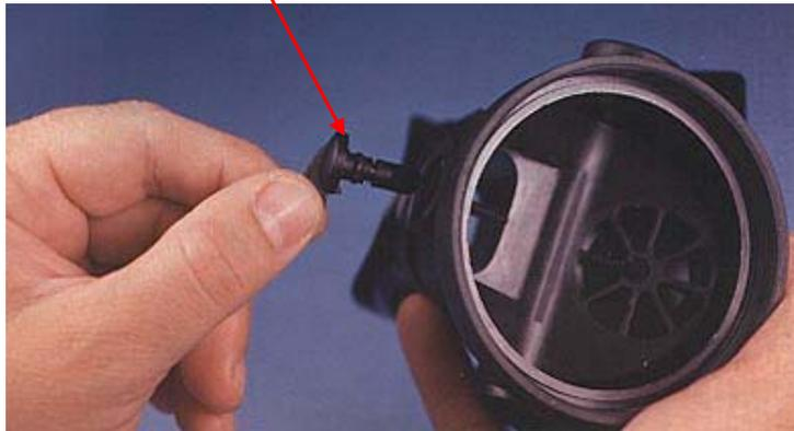
**Using needle nose pliers replace Clip RG1422**
