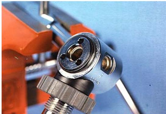
12) Lubricate and install “O” ring on the first stage housing for the turret
