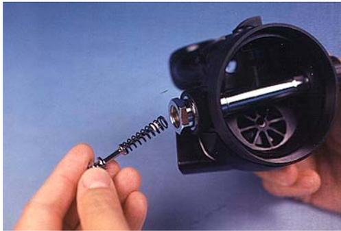
**Remove the Inlet Tube RG1407 and the Spring RG1403**
