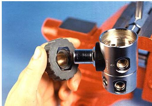
22) Using a 19mm Socket wrench loosen and remove the Din Connector and Saddle
