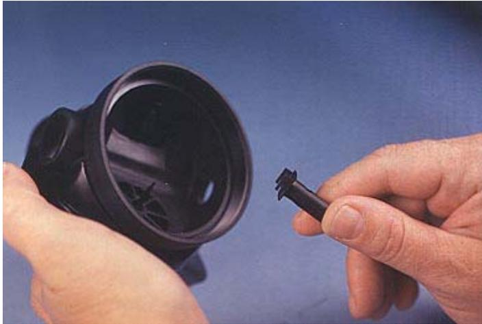
**The Deflect tube RG1422 can now be removed take note of the orientation before removal. Small opening faces the Diaphragm**
