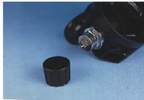
11) using a 3/4 inch wrench remove the Packing nut
