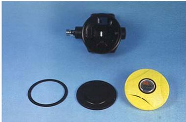
6) Remove the retainer ring and diaphragm
