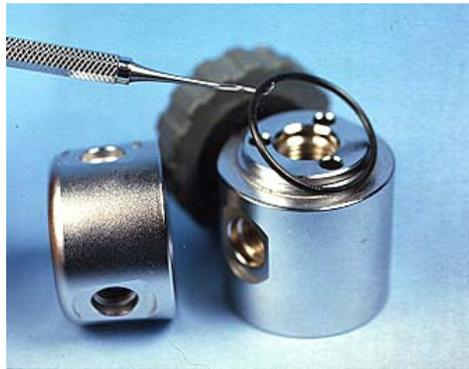
17) Remove the Turret and corresponding large “o” ring
