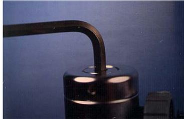
6) The Intermediate pressure is to adjusted to 140 psi +/- 5psi at high pressure
