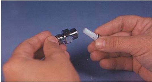
**Lubricate and Install new “o” ring RG1411 on *New Orifice RG1412***
