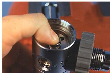
24) Install the Diaphragm ( Make certain that the diaphragm is seated below the threads and is in contact with the seating surface
