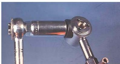
Apply One (1) drop of Locktite to the threads before screwing DIN connector into Housing
