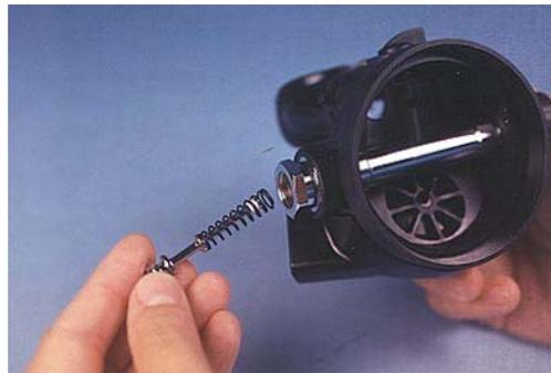
**Replace the Inlet Tube RG1407 and the Spring RG1403**
