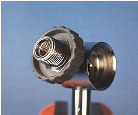
9) Lubricate and install “O” ring on the top of the din wheel lockdown screw
