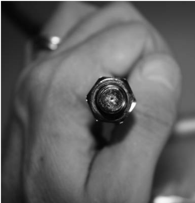
Male end opening of high pressure hose
