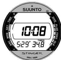
Fig. 2.7. The Stopwatch displays hours, minutes and seconds.
