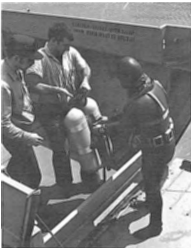
5. The diver has his hood on and with the aid of a tender is preparing to put the SCUBA on. Shoulder straps have been adjusted and tied for quick-release.
