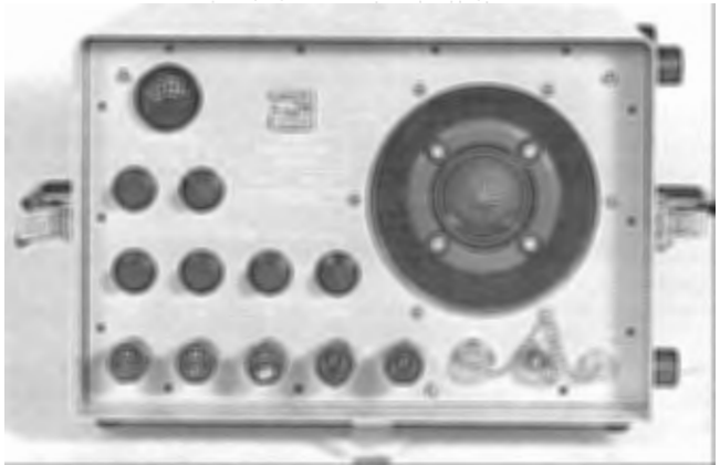
Figure 6-34 Model 2 Diver's Intercommunication System
