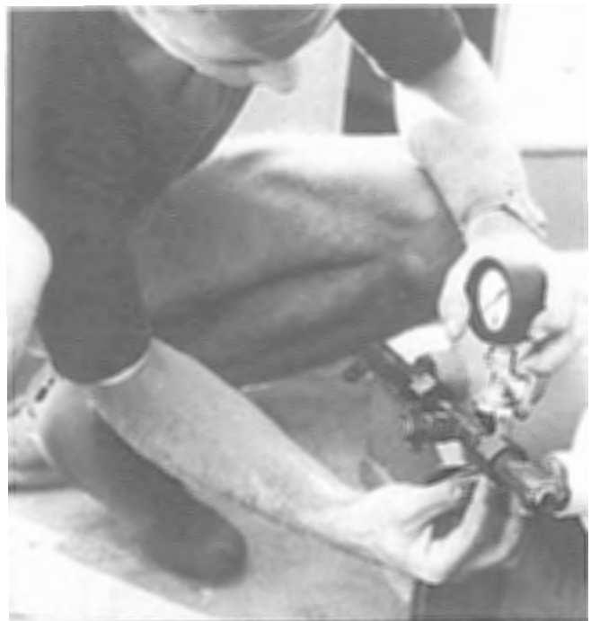
Figure 5-29 Gaging SCUBA cylinders
