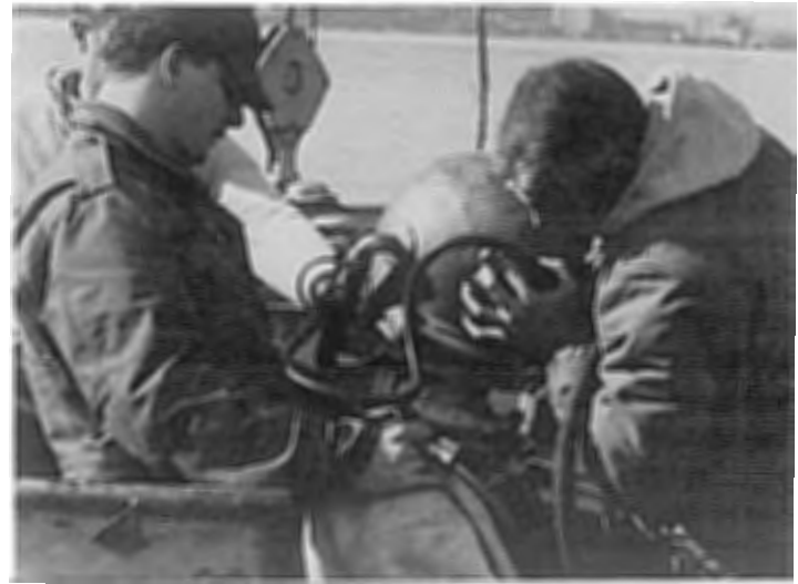
M The helmet, with face plate open, is carefully lowered over the diver's head and properly aligned.
