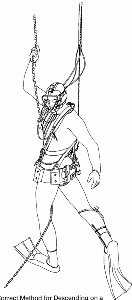
Figure 6-40 Correct Method for Descending on a Descending Line
