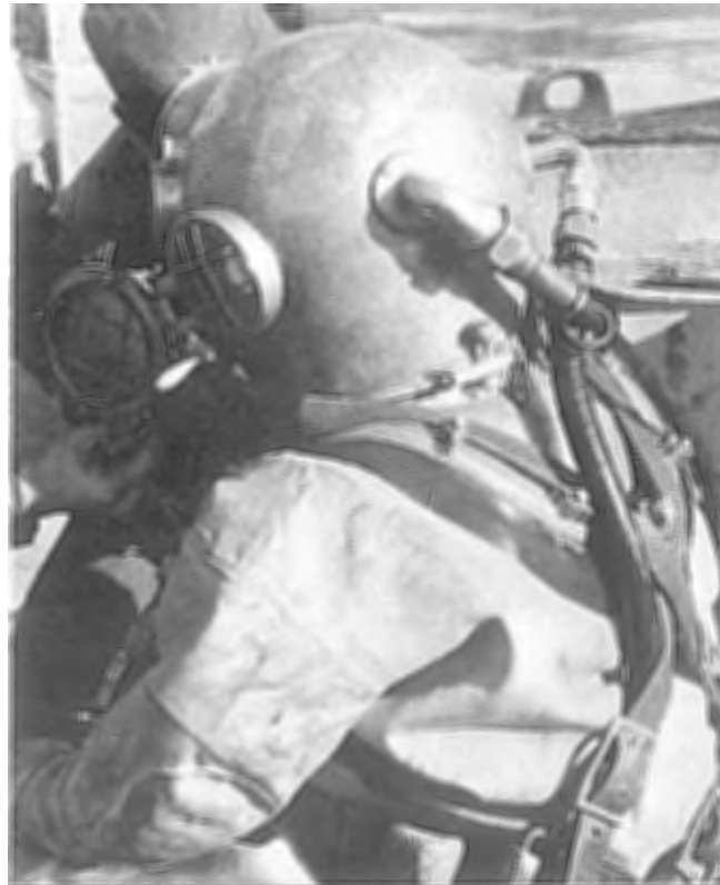
Figure 6-13 Air hose, communications cable and fittings shown properly secured to diver.
