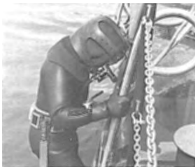
Figure 6-15 Lifeline, air hose and pneumofathometer (behind right hand) in use for lightweight diving.
