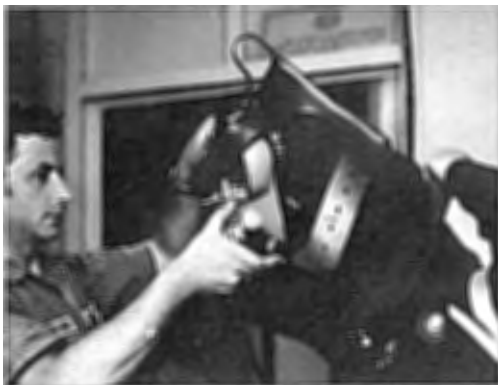
H With the mask air supply on, the tender aids the diver to pull the mask over his head.
