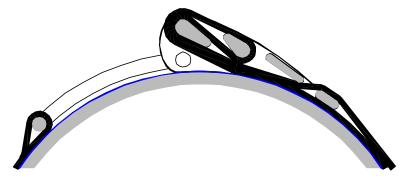
Rotate the cam closed. It should require a fair amount of force, but don't over-tension. Ask a dive professional if you are not sure of proper tightness. Aggressive jerking on harness can test for secure assembly. Don't get body parts caught in the cam; it can cause serious injury. Secure the end of the webbing with Velcro or lace through a keeper.
