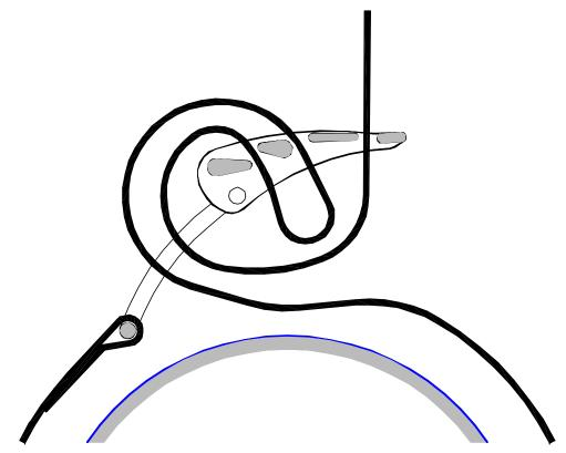
Pass the end through the end slot from back to front
