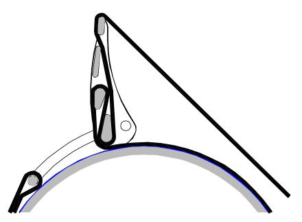
Position the BC on the Scuba cylinder with the band perpendicular and pull the slack through so the band is snug when the buckle is approximately vertical.
