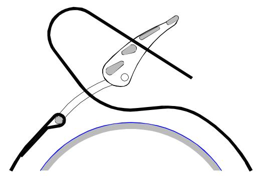
Pass the end through the middle slot from front to back.
