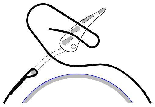
Pass the end through the inner slot from back to front
