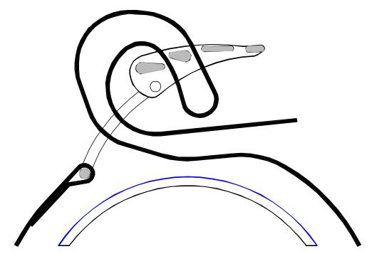
Pass the end through the bale between the buckle and webbing from front to back
