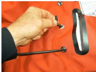
**#3** Thread loose end back through adjacent grommet inside of wing.
