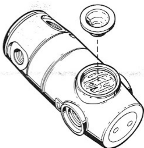
Fig. 17 - Secondary Diaphragm Installation
