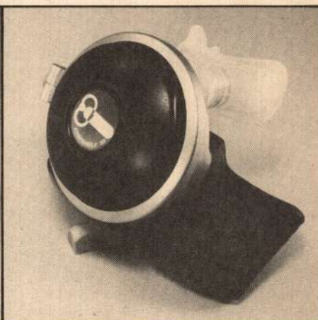
From left: Diagram of Conshelf 30 second stage; first stage; second stage, assembled. The first stage has one 7/16 inch diameter high pressure port and four 1/2 inch diameter low pressure ports. All ports are angled down 45 degrees. The second stage has an oversized exhaust valve and tee, silicone rubber mouthpiece and diaphragm, and a brass case with a polyester powder coat on the front.
