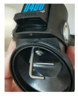
Additionally, the lever was lengthened (D350), and then thickened (D400) to improve mechanical advantage and smoothness of lever action.
