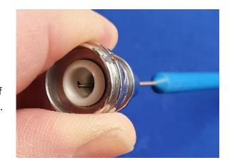
The static o-rings that seal the orifice to the housing are spec'ed by Scubapro as AS568 5-179 duro 70. However, this is roughly a 1x6mm oring, and the lands in the techno-polymer orifice measure 8.37mm diameter. A 1x6mm therefore requires significant stretch, and I am surprised at the specification. A 1mm x 7mm duro 70 fits quite well and is my choice, but as a static oring it probably makes little difference either way, as long as you can insert the orifice and it seals in the housing.
