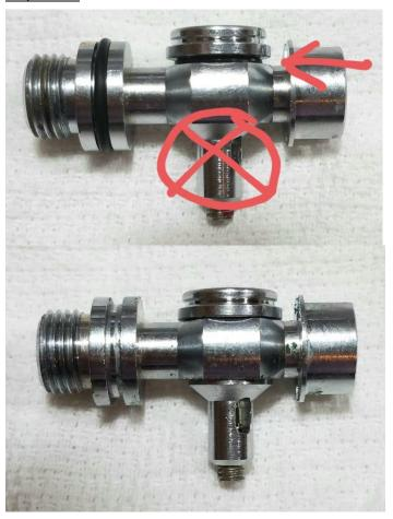
Inlet Tube – The inlet tube comes in two iterations, with a noteworthy consequence. It is critical that the housing is fully seated in the inlet tube before pressurization to avoid leaks.
