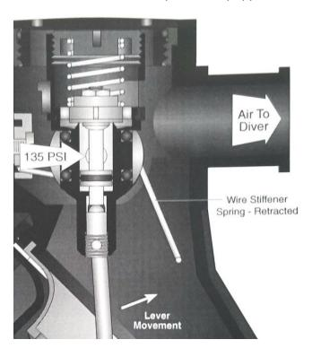
Spring fatigue is a factor in these old regs, and it is not uncommon to find a spring pad which is fully screwed in, and yet the valve still freeflows. After restoring the knife edge, it is usually possible to shim the poppet spring with a graphite impregnated washer from McMaster-Carr (PN 91545A270) and obtain enough spring pressure to seal.
