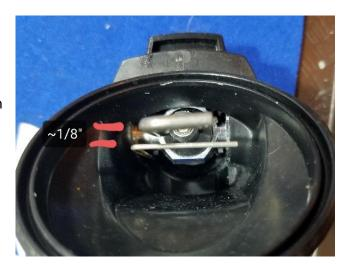
Next, using a custom tool, the pins in a Scubapro tool, or a small pin face spanner, unscrew the cap (1) on the top of the case. The Scubapro tool is by far the worst tool for the job, as it is easy to rock one pin up and out of the hole, scratching the cap as you rotate the tool. Using thumb pressure, it is easier to keep a face spanner seated.
