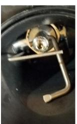
Because of this problem, the D400 was redesigned, placing the leg of the lever on the <u>left</u>, where the spring end will not trap it.
