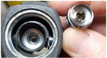
One consistent characteristic, however, is the fragility of that knife edge. Used regulators almost <u>always</u> show damage, such as these examples:
