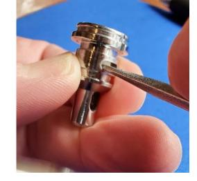
Then, using a straight blunt pick, carefully engage the side of the orifice from below through the stem of the housing, and carefully push up.
