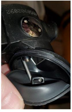
Examine the diaphragm assembly, but do not attempt to disassemble it. The plastic cone of the exhaust retainer (28) that fastens the pieces together is essentially a single use item, and replacements are as rare as hens' teeth.
