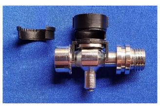
The gate is adjusted using the forked end of a brass spade, or similar long narrow tool, to engage one side or the other of the collar. Max flow is with the gate edges symmetrically at the edge of the oval airflow hole in the aspirator. The D400 will easily freeflow with the mouthpiece off and the aspirator centered.
