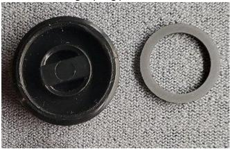
Alternatively, if you have a late model D400 with a perforated spring adjuster and separate white spring pad, flipping the spring pad over reveals a thicker side that effectively shims the spring using the pad itself.
