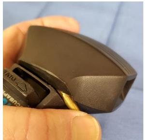
Once the rubber cover softens, insert the spade in the front of the case at a 45 degree angle to the gap between the case at the bottom of the predive switch. Pry up the thick top of the cover front.
