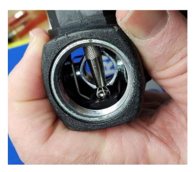
With the parts loosely connected (and with pressure maintained on the switch and oring), switch to your screwdriver for final tightening. As with the grabber, insert the screwdriver through the mouthpiece tube, with the switch maintained in the uppermost predive position. This brings the screw head into view from behind the inlet tube.
