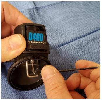
NOTE: if heavily corroded with blue-green verdigris, this hex screw can be nearly impossible to remove. If the 3/32" hex key is a sloppy fit, you may strip the hex if significant force is applied. In this case, a 2.5mm metric hex may fit more tightly and grip the hex screw without stripping. But there is an additional problem: the housing tries to twist when you unscrew the hex, which is why pressure is applied to the housing while you unscrew.
