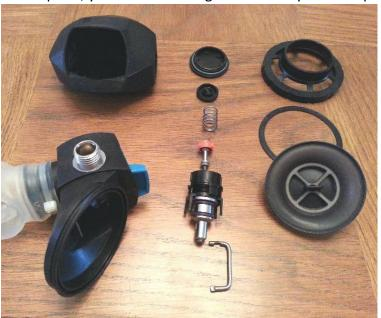
Removal of the inlet (32) and predive switch (34) is not necessary unless significantly corroded or leaking. If you do not intend to remove the inlet or Pre-Dive switch, skip to "Cleaning" below.
