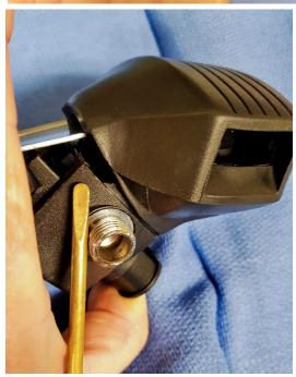
After prying up the front corner of the cover, using your third hand, slip the flat blade of a cheap spoon handle, or the bowl of the spoon itself into the gap between the case and the thick cover. Make sure the PreDive switch is in "Pre" to be up and out of the way. Pry the spoon/handle back until you can see the top edge of the diaphragm cover ring. The smooth "shim" of a spoon handle keeps you from gouging the case.
