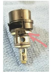
The way to do that is to insert a 3.5mm hex key in the hose inlet of the regulator, and manipulate it until the hex key passes into the inlet tube and <u>through **both** sides of the housing</u>.
