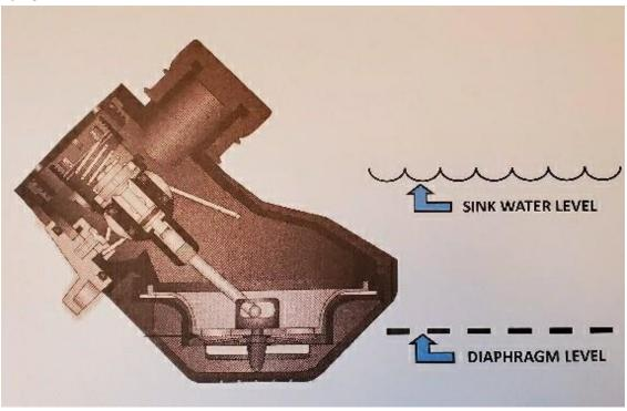
Cracking effort can be fairly precisely estimated by the depth to which the regulator is submerged when a slight hiss begins.
