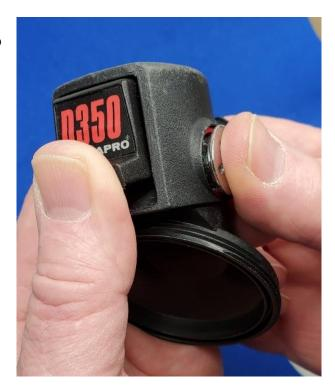
Then remove the retainer completely, along with the static o-ring (18) underneath. Carefully press on the visible end of the inlet, taking care not to pinch your finger on the sharp corners of the alignment ridges in the case (ask me how I know).
