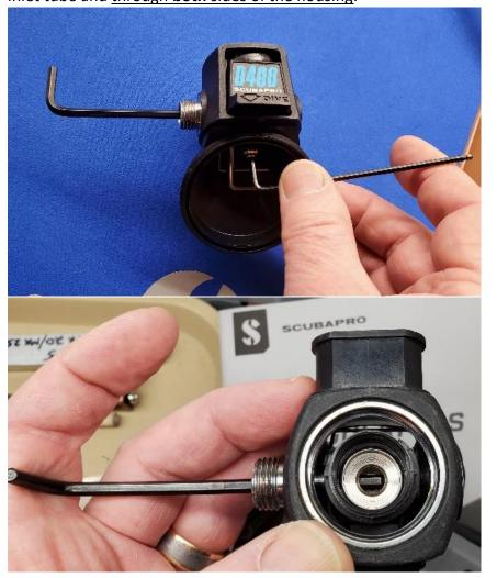
This only works with D-series regs that do not have the techno-polymer knife edge, as that last model has side slots instead of holes in the housing, and will still twist.
