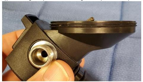
It is not optimal to eliminate all lever slack. When the diaphragm is attached and the cover ring screwed down, a lever that is too high will be displaced by the linkage loop even before a breath moves the diaphragm.
