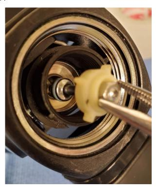
Balance the poppet spring centered on the top of the poppet and add the spring pad (with or without an aftermarket graphite impregnated shim). When you are sure that the spring pad has engaged the spring in its center, screw the spring pad into the aspirator until it is flush with the top edge, and then 1/2 turn more. This is your preliminary tuning position.
