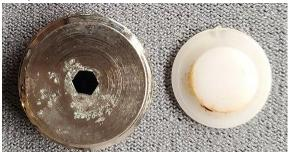
Finally, the Air1 regulator came with a poppet washer to decrease spring binding. If you have access to the rare SP part 01.060.100, that can be used to shim the poppet as well.
