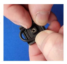
Here is the difficult part: with the switch capturing the o-ring on at least three sides, with your third hand carefully pick up the case and press the switch <u>firmly</u> against the front of the case. At this point, if you aren't using the square o-ring, you can use the forked end of a brass spade to push the bulging top of the 2-116 o-ring under the switch edge into the land, and with firm pressure on the switch, the o-ring will remain in place, trapped between the case and the switch.
