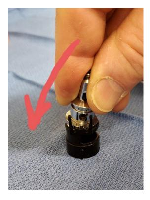
Now add the VIVA collar (aspirator gate) to the aspirator, with the larger diameter toward the top of the assembly. Confirm correct orientation by feeling for clicking as the collar is rotated around the aspirator. Position the collar in the fully open position, with the space between the collar arms centered over the hole in the aspirator front.
