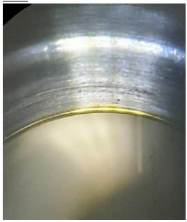
With a restored knife edge, it will be essential to thoroughly rinse after every day of salt water diving, and perhaps repolish out any corrosion every 1-2 years. I will post on restoring a D-series knife edge in an upcoming thread.
