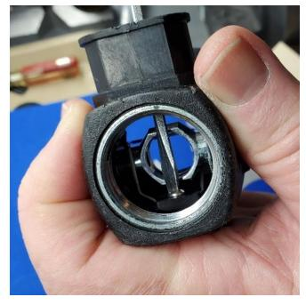
where you set it. Firm tightening will bring the back of the retainer into contact with the switch mount for the screw, so that net tension is provided solely by the compressed o-ring, and not by additional tightness of the screw. If switch action is sloppy with your particular switch, consider reinstalling with a 2-117 oring, though this is only rarely needed.
