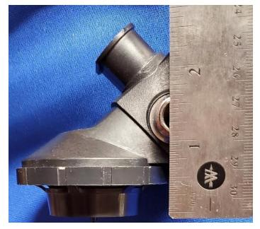
So, adjusting cracking effort is a straightforward (if slow) matter of repeatedly setting the spring pad position, attaching the top cap, pressurizing the reg and submerging it until you can just hear the reg begin to hiss. This regulator, tuned to 0.8"WC, has just begun to hiss as the water level in the sink rounds the back of the case.
