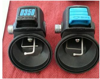
In rare cases, the lever can get caught behind the spring, and the regulator will freeflow when the switch is placed in the Dive position as the spring pulls the lever back with it.
