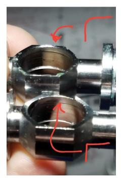
Thus, the use of a 75 Duro aftermarket o-ring may prompt it to extrude along the radius. As discussed below, a harder Durometer 90 o-ring does not seem to have this problem. Note that the original o-ring from Scubapro (01.050.147) was spec'ed at Shore A85. However, if your inlet has a sharp corner on the land, either a Duro 75 or 90 seems to work well in sealing the housing.
