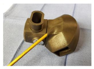
First, slip a brass spade under the cover in back. Sliding it sideways will break any seal.
