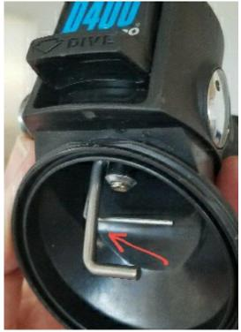
To determine how much to bend the spring, sight along the axis of the housing and determine how much separation there is between spring and lever with the regulator positioned mouthpiece down. Note that with the mouthpiece up, normal lever slack will allow it to fall forward away from the spring and you will have an incorrect (excessive) estimate of spring shortfall. Write down the amount of bend the spring will require.
