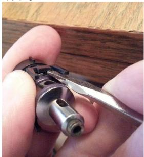
Instead, it is easiest to pop the aspirator off the housing by pushing with your thumb against the <u>side</u> of the aspirator, while applying counterpressure against the stem of the housing where the hex key lives. Pushing from the back or front of the aspirator risks breaking the little loop of plastic that engages the housing at the front. The side of the aspirator is the strongest location for pressure.
