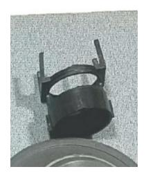
The aspirator is usually <u>tightly</u> fitted to a groove in the housing. Do NOT try to remove the aspirator by prying in this fashion:
