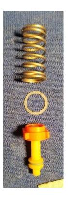
There is yet another workaround, however. You can use reduced Intermediate Pressure to get a seal. Higher IP will tend to creep around the knife edge/poppet seat interface due to the straightforward physics of spring pressure in pounds divided by knife edge area in sq. in.
