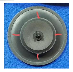
Carefully lift one side of the diaphragm, and while watching the plastic linkage loop (26) that engages the lever underneath, slide the loop off the lever. The direction in which to slide the linkage differs between the D300/350 and the D400 (slide right with the 400; slide left with the 300/350).
