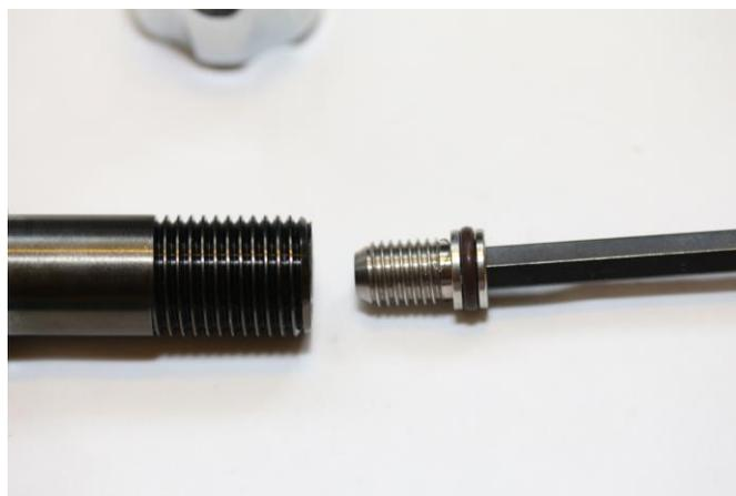
Remove the LP seat (ITEM 12) from the piston. Remove the piston from the balance chamber.
