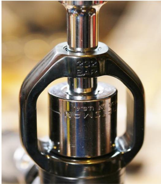
Use the  $\frac{3}{4}$  socket and 3-inch extension to loosen the yoke retainer (ITEM Y4).
