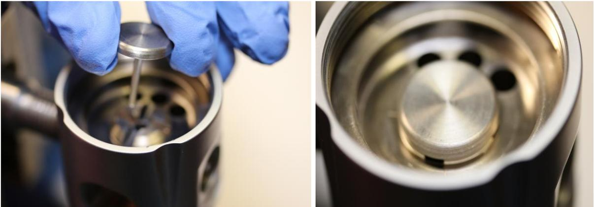
Next install the diaphragm (ITEM D28/Y26). The diaphragm is most easily installed by bending it slightly and inserting it into the groove below the threads.
