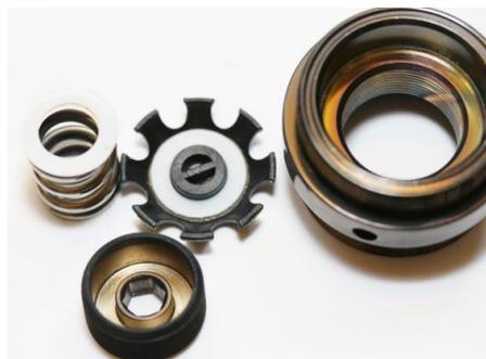
Remove the diaphragm (ITEM D28/Y26), and valve lifter (ITEM D27/Y25).
