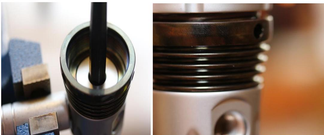
Take the turret/IP Cap assembly and screw it on to the main body that is secured in the vise after you have installed the body/turret O-ring (ITEM D13/Y11). Tighten with the pin spanner so that there is no gap between the two components and the connection is secure.
