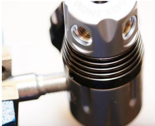
Using a number 5 pin spanner, remove the turret assembly by loosening the IP Cap (ITEM D21/Y19) . Once loosened, unscrew it from the main body. If difficult to remove refer to page 11.
