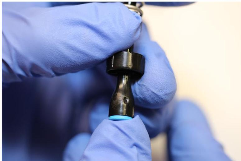
Set the spring on the shoulder of the balance chamber. Holding the balance chamber vertical, place the piston through the spring and into the balance chamber. Push down gently on the piston to make sure that it moves smoothly.
