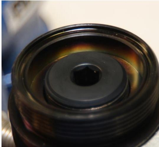
Stack one plastic washer, the main spring, second plastic washer, and the spring seat in the main spring adjusting screw as seen in the following image.
