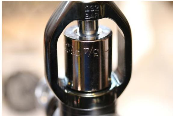
Following torquing the assembly, install the yoke knob (ITEM Y1). It is highly recommended to apply a thin coat of lube to the threads on the knob before screwing it in.
