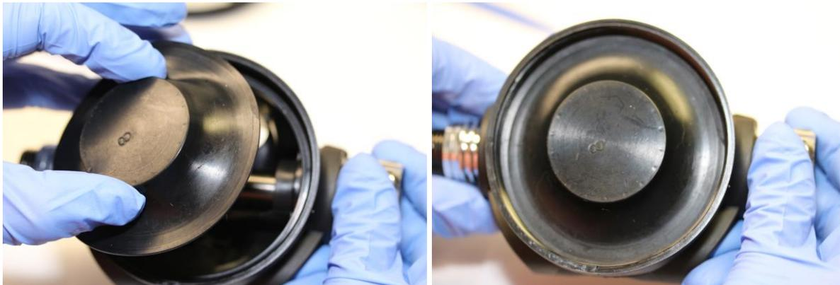
Install the faceplate. This completes the assembly of the 2<sup>nd</sup> stage. Final adjustment and testing is covered in the next chapter.
