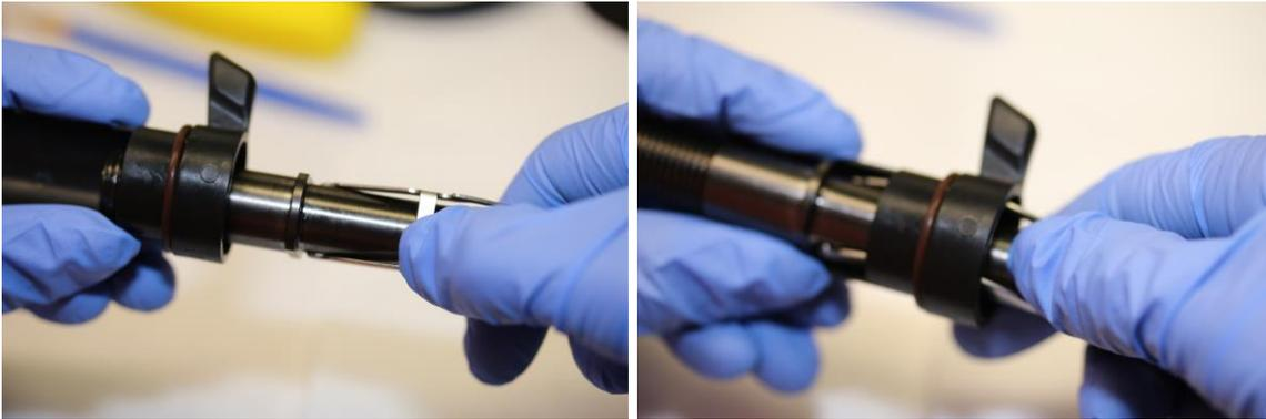
After having installed the deflector knob on the air barrel, slide the assembly into the second stage case. You will need to hold the lever down to ensure smooth insertion and to avoid damage to the lever.
