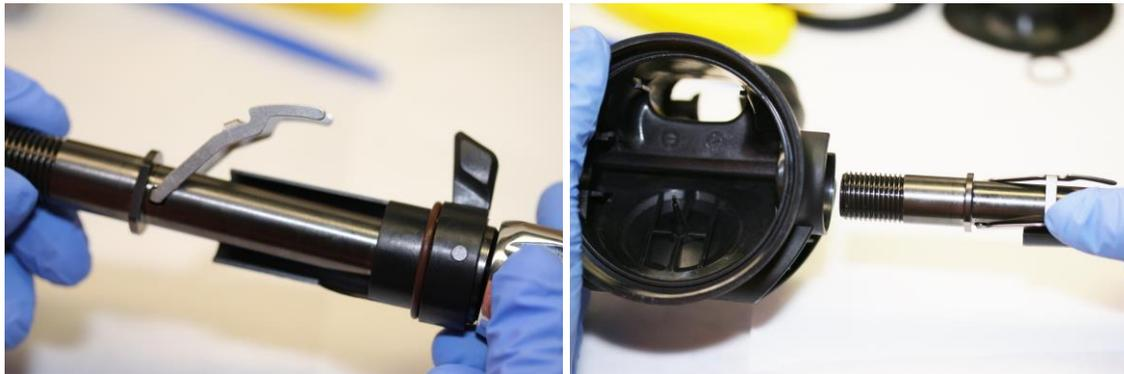
Slide the assembly in until the flat flanges of the air barrel fit into the locking lugs of the case as shown.
