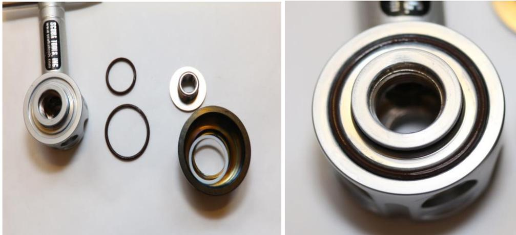
Taking the turret (ITEM D24/Y22), swivel retainer (ITEM D19/Y17), Teflon washer (ITEM D20/Y18), and two O-rings (ITEM D22 and 23/Y20 and 21), lubricate the O rings and place them in the grooves on the turret. Take the IP Cap (ITEM D21/Y19) and place it on the turret. Make sure that it rotates freely and is seated. Install the Teflon washer in the turret body. Using the 8mm hex wrench, tighten the swivel retainer to 150 inch pounds.
