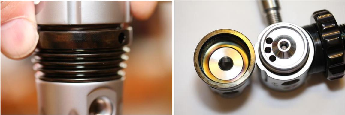
Using an 8 mm hex disassemble the turret to reveal the Teflon washer (ITEM D20/Y18), Swivel Retainer (ITEM D19/Y17), turret (ITEM D24/Y22), and the two O rings (ITEM D22 and 23/Y20 and 21) that seal the turret.
