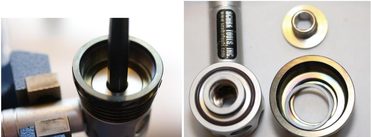
Remove the O rings from the turret and place them with the old parts to be replaced.
