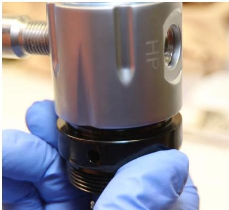
Using the #6 Pin Spanner tighten the diaphragm clamp assembly until there is no visible gap between the retainer and the body. *Due to the nature of the soft diaphragm, there is no torque specification. Make sure there is no gap and the connection is tight.*
