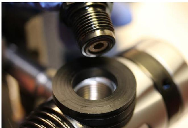
Taking the torque wrench and crow's foot or 13/16 deep socket, tighten the DIN housing to 230 inch pounds.
