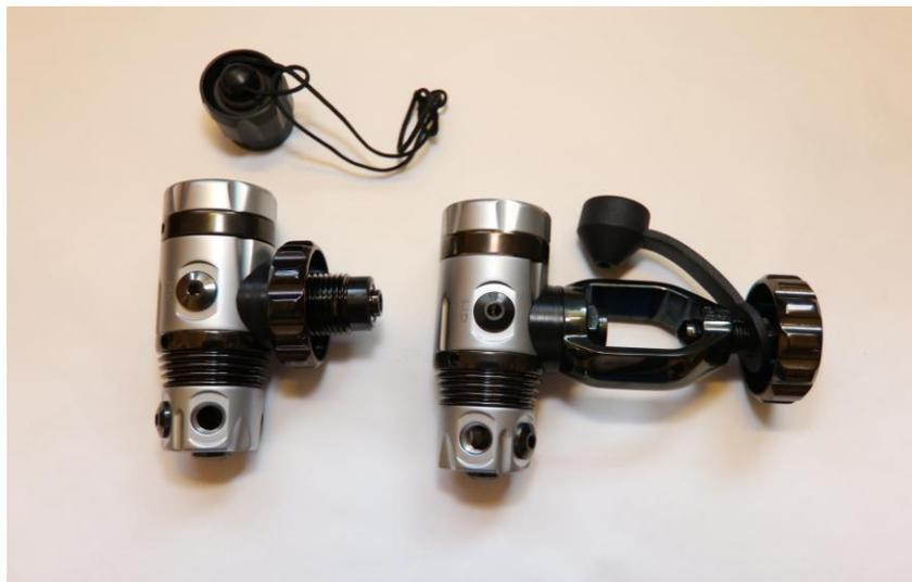
**Second Stage Main Housing Integrity** – The integrity of the second stage main housing (ITEM 1) should be determined by looking for any obvious signs of damage. Scratches, gouges, missing parts, damaged exhaust ports, or loose cover retainer, or damaged cover may be indications that housing integrity has been compromised.
