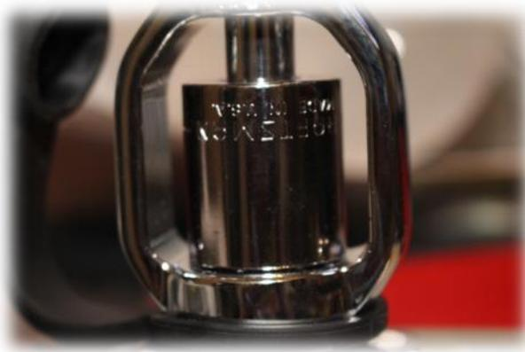
Remove the yoke retainer.
