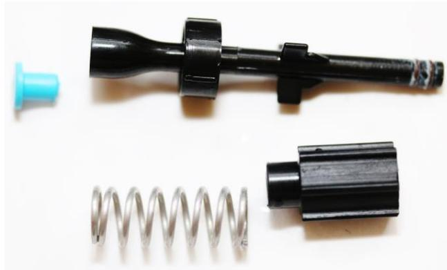
Remove the two small O-rings (ITEM 14) on the piston. Clean and dry the piston, balance chamber, and spring. Remove the O-ring (ITEM 6) from the deflector knob (ITEM 7). Clean and dry the knob.
