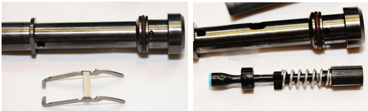
Inspect and clean the adjust tube/lever assembly. Set it aside. Remove the O-ring (ITEM 8) from the air barrel (ITEM 9) and set it with the other used parts to be replaced. Clean the adjust knob (ITEM 18) with a degreasing agent and water, deal with any corrosion as previously noted, rinse and dry. Place them in the cleaned parts area.
