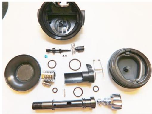
This completes the disassembly and cleaning of the second stage
