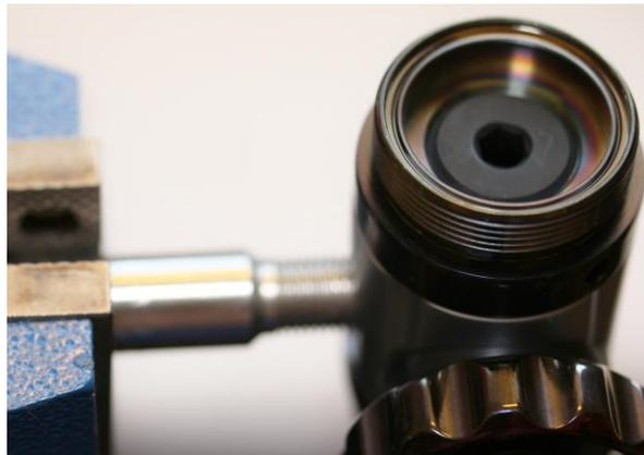
Unscrew the adjustment bolt at least 3 full turns to remove pressure on the mainspring (ITEM D31/Y29).
