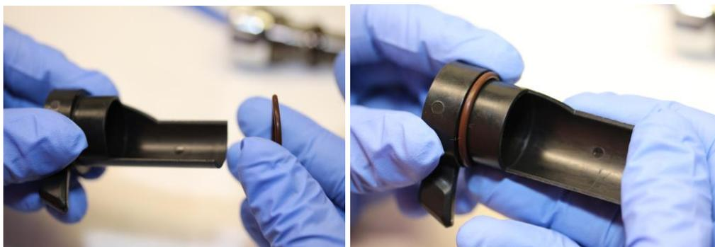
Holding diaphragm lever down, slide the deflector knob assembly over the air barrel from the orifice side. Take care not to bend the main diaphragm lever.
