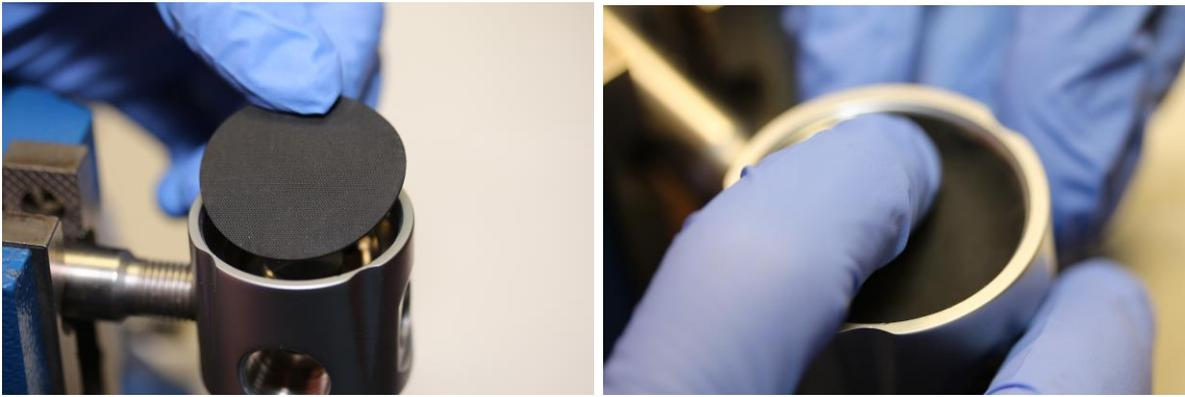
The diaphragm may require the use of a blunt brass pick. Work one side in and as you press the diaphragm into place, work it into the groove all the way around the body. **DO NOT WRINKLE OR TEAR THE DIAPHRAGM!**
