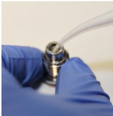
Lightly lubricate the balance plug outer O-ring (ITEM D17/Y15) and slip it into place below the threads and into the space around the bottom of the balance plug. Set the
