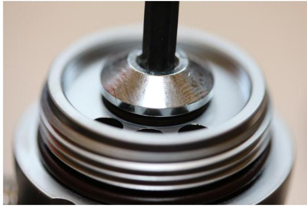
Having loosened the plug, remove the 1<sup>st</sup> stage from the vise and turn the body diaphragm side up. Remove the balance plug from the main body. Remove the turret O-ring (ITEM D13/Y11) from the body.
