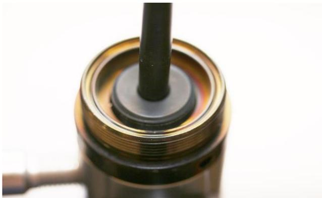
Using the Pin Spanner, loosen the clamp (ITEM D33/Y31). Do not remove it entirely yet! If difficult to remove refer to page 11.
