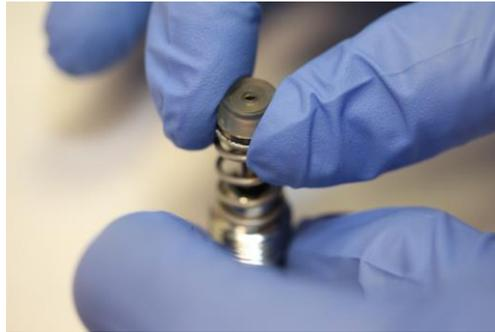
Press the seat gently a few times to ensure that it moves freely through the inner O-ring.
