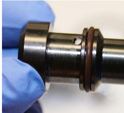
Insert the piston assembly into the air barrel as shown. Note orientation of the hole.
