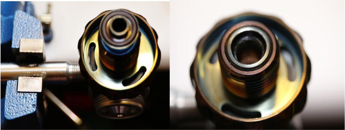
Remove the DIN wheel (ITEM D5) and set it aside with the DIN retainer.
