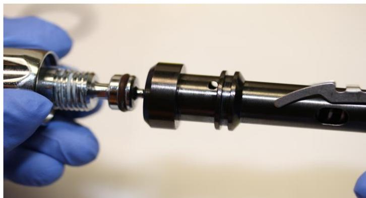
Once it is started screw the assembly in. The lever should start to rise. If it does not go back and repeat the piston removal and assembly steps.
