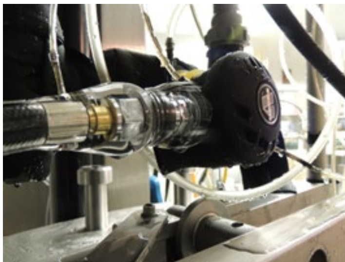
Figure 5. Ice formation on air supply line to second stage regulator
