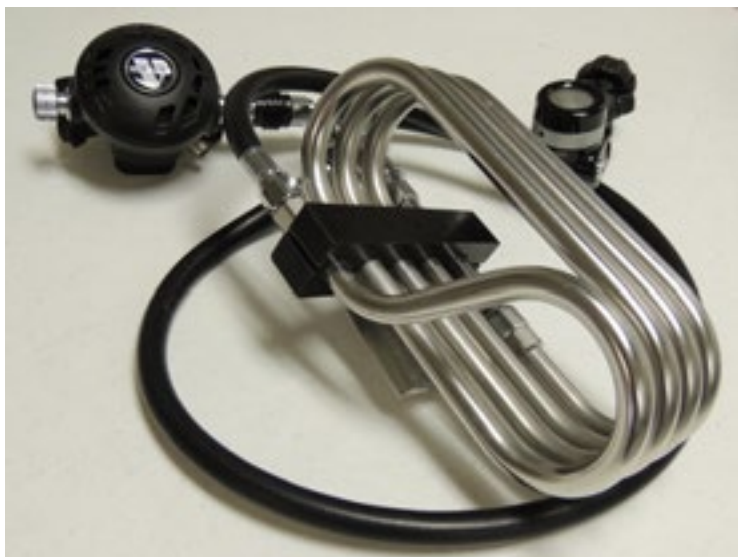
Figure 10. Kirby Morgan Thermo Exchanger (TE)
