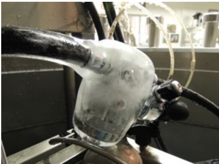
Figure 7. Extreme First Stage icing event.
