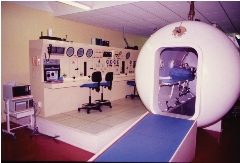
Figure 5 Multiplace hyperbaric chamber. The chamber is pressurized with air, and delivery of 100% oxygen may be achieved either by the use of a hood sealed around the neck through which oxygen free flows or by a demand valve and oronasal mask.
