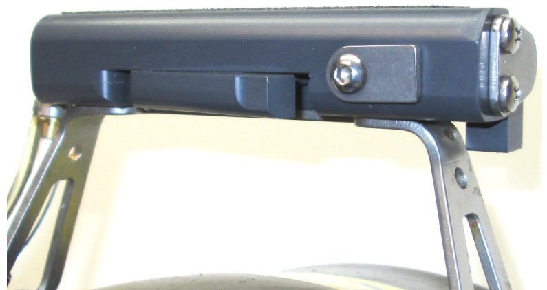
Figure 8 - Lock tab 180° from trigger
