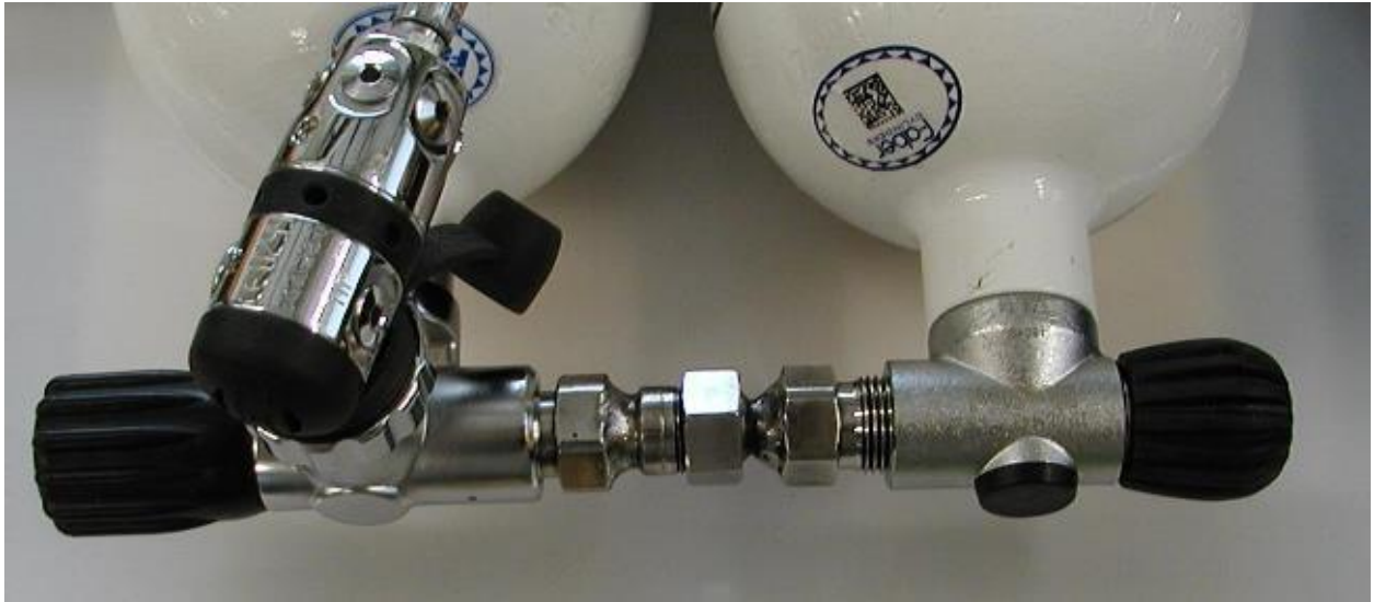
Figure 27. Custom doubles manifold for bail-out bottles for surface supplied diving.
