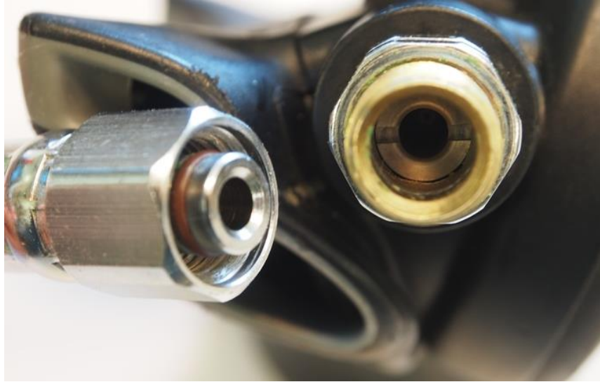
Figure 10. Hose connector to the second stage regulator is a dynamic seal. Look closely and you can see the brown O-ring in the groove under the lock nut.
