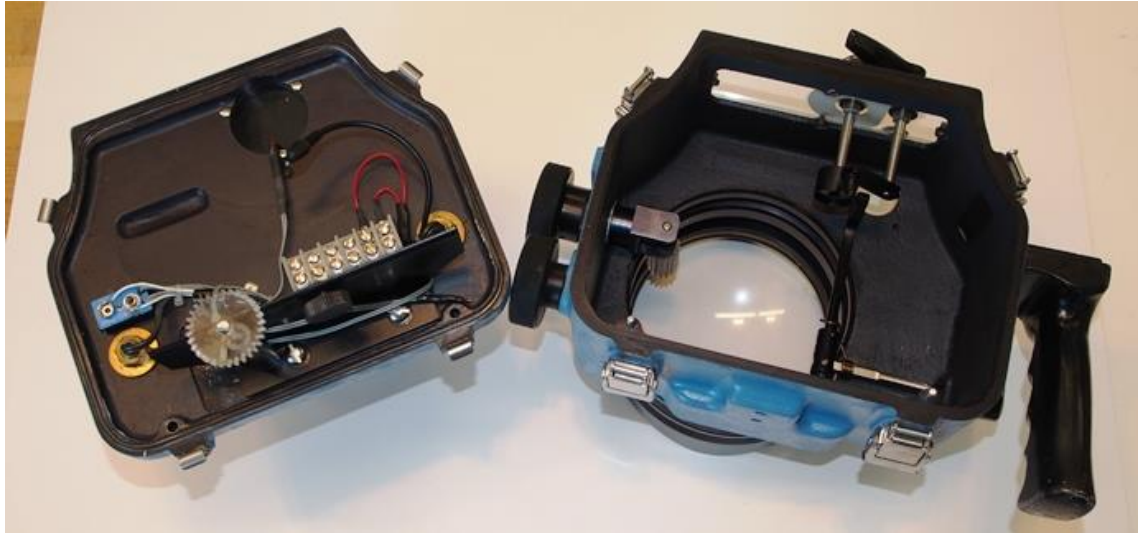
Figure 6. O-ring grooves don't have to be round. This image of is an underwater camera housing. This is classified as a static pressure-seating face seal O-ring.
