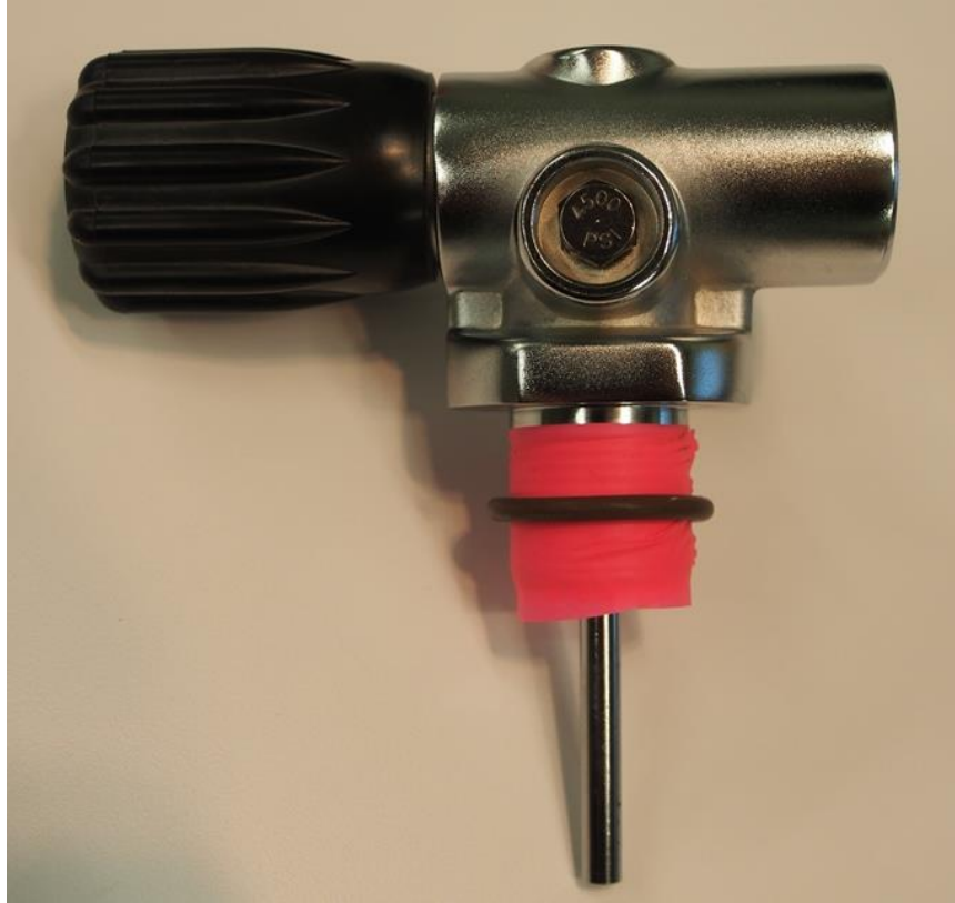
Figure 17. O-rings can be protected from thread damage on Scuba cylinder valves with adhesive-free Flagging Tape.
