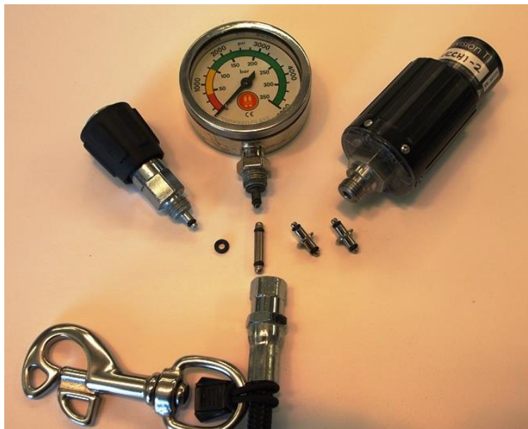
Figure 11. The standard HP (High Pressure) hose connection that was originally designed for SPGs are also used for AI (Air Integrated) dive computer adapters and wireless transmitters for AI wrist-mounted computers.
