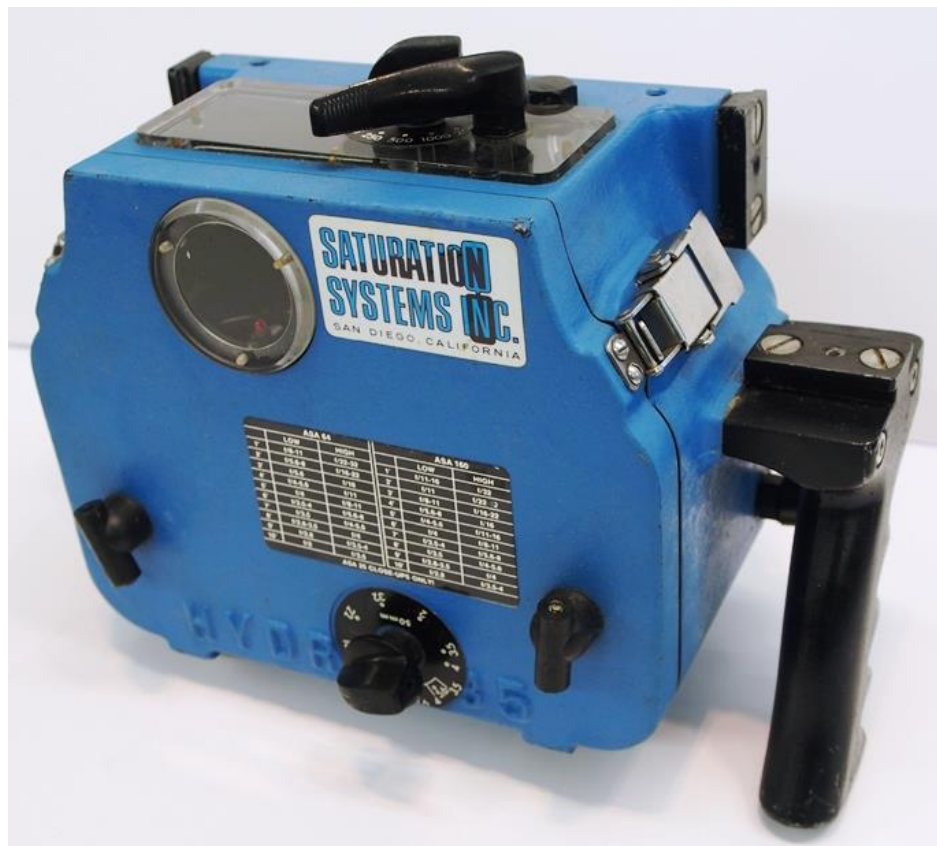
Figure 7. Pressure-seated O-rings like this one don't require robust clamping mechanisms because the pressure does the work. The four small spring-loaded latches are all it takes to compress the O-ring enough to make the initial seal.
