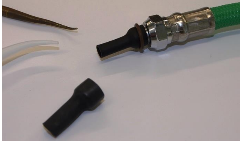
Figure 16. Shrink tubing makes excellent thread protectors for installing O-rings on SAE J1926 straight thread boss connections used on first stage regulators.
