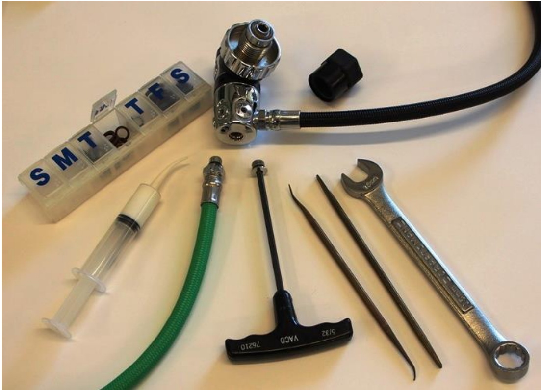
Figure 2. You can repair most leaks with some spare O-rings, a removal tool kit, a wrench or two, and some lubricant.
