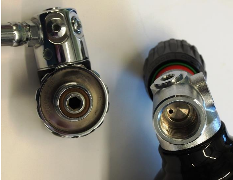
Figure 4. The first O-ring that divers learn to use is usually the stage regulator connection to the cylinder valve. This image is of a DIN connector.
