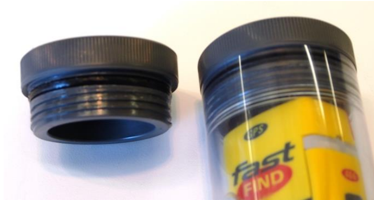
Figure 8. This PLB (Personal Locator Beacon) housing has threaded caps at both ends with static piston seal O-rings. You can see the compression of the O-rings through the clear plastic tube.
