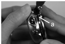
Fig. 166 - ALIGNMENT OF FRONT/BACK
