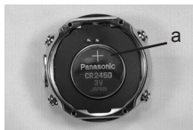
Fig. 163 - BATT INSTALLED
