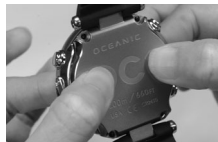
Fig. 167 - PRESS FRONT AND BACK TOGETHER
