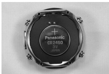
Fig. 165 - BATT INSTALLED
