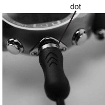
Fig. 159B - PCI CABLE (turn dot to 1 o'clock)
