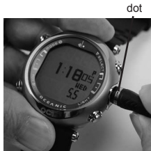
Fig. 159A - PCI CABLE (insert with dot at 12 o'clock)
