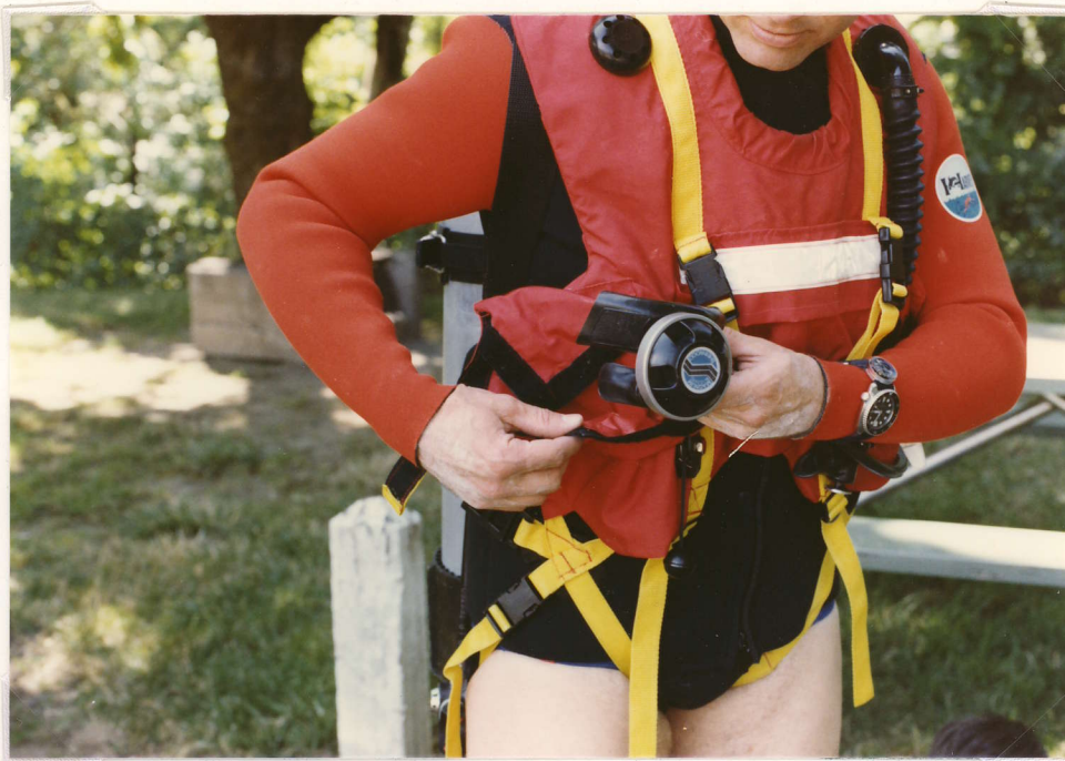
Photo #13: The Octopus/weight pocket can be used for an octopus second stage of a diving regulator in the following manner. First, open the pocket up and insert the second stage. Note that if the regulator is on a long hose, it is recommended that it go in upside down. This prevents free flow and allows easy use by a distressed diver. On the long hose it can still be used by the donor diver in case the recipient diver uses the primary second stage out of the donor's mouth.
