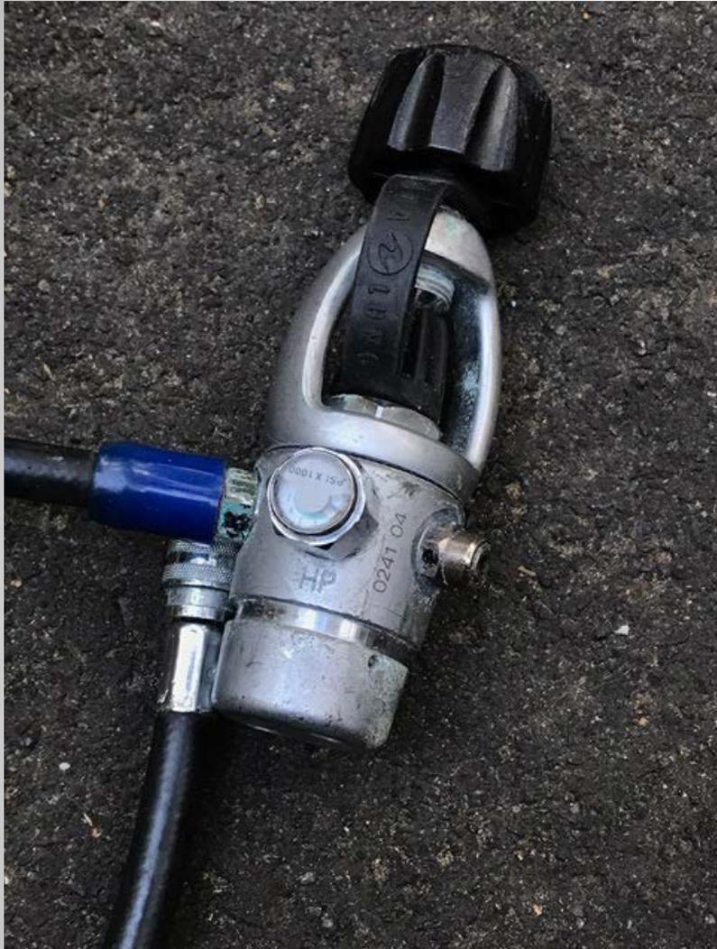
First stage for Argon bottle, with very tiny pressure gauge
