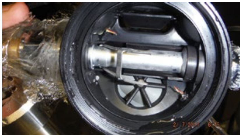
Figure 2. Regulator that experienced free flow after ice formation
