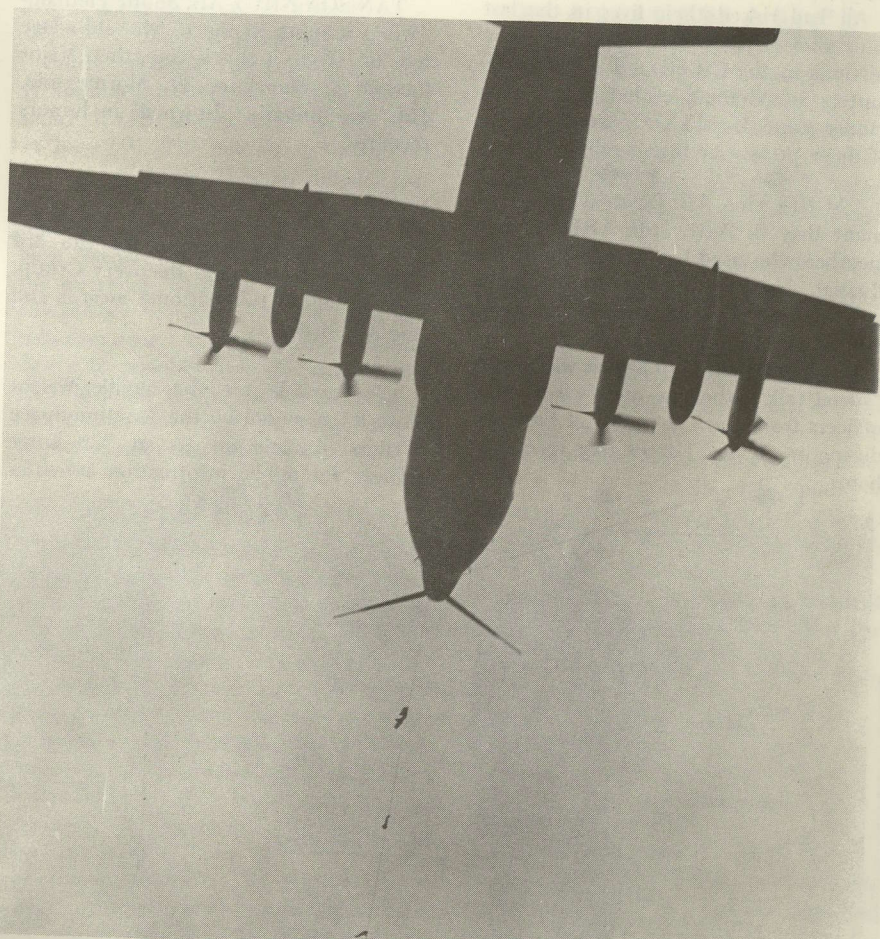
AN HC-130 ENGAGES THE LIFT LINE to begin a surface-to-air recovery. This photo was taken from the deck of the prime recovery ship following recovery operations for Apollo 8. The package recovered contained films of the recovery.
