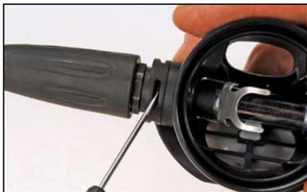
22. With the control Knob still rotated fully counterclockwise complete the fine adjustment as follows:
