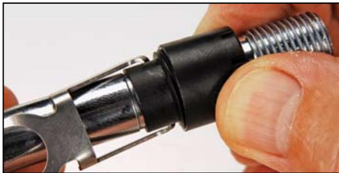
7. Place a lubricated new O-ring (18) on the Stem (19) and insert the Stem into the Adjuster Body (17). Use a 1/8" hex key to fully seat the Stem inside the Adjuster Body. Do not over torque. Just tighten until you feel it stop. When fully seated the Stem should project from the Adjuster Body by about 1/16 ". Place a lubricated new O-ring (16) on the Adjuster Body. Set subassembly aside for later insertion onto the Valve Body.
