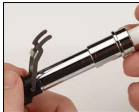
10. Insert the Adjuster Body (17) into the Valve Body (9) threading clockwise just until thread engagement starts. Place the control Knob (20) onto the Adjuster Body and continue threading the adjuster Body into the Valve Body until the groove in the Adjuster Body is centered in the rectangular hole in the Valve Body.
