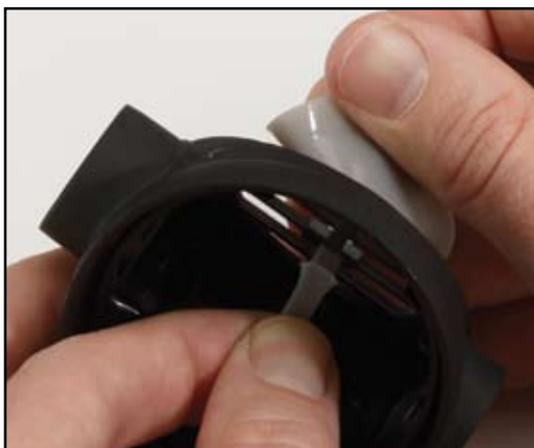
13. Remove the Adjustment Sleeve (2) from the Valve Body by rotating it counterclockwise. Remove O-ring (3). Set both parts aside for cleaning, inspection and reassembly.
