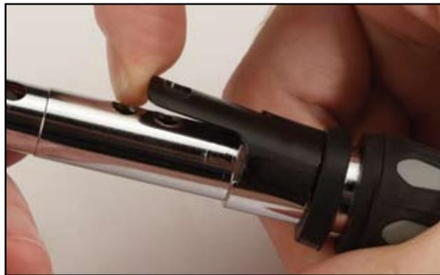
17. Remove the Ring Seal (6) by moving it toward the threaded end of the Valve Body.
