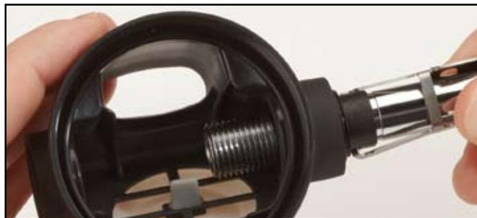
15. Insert lubricated O-ring (29) and install the Clip (35) over the Valve Body between the Adjustment Sleeve and the threads of the Valve Body. Install the Retaining Nut (28) and tighten until snug.
