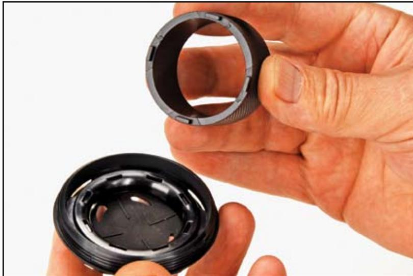
7. Remove the Diaphragm (**26**) and set aside for cleaning and reassembly.
