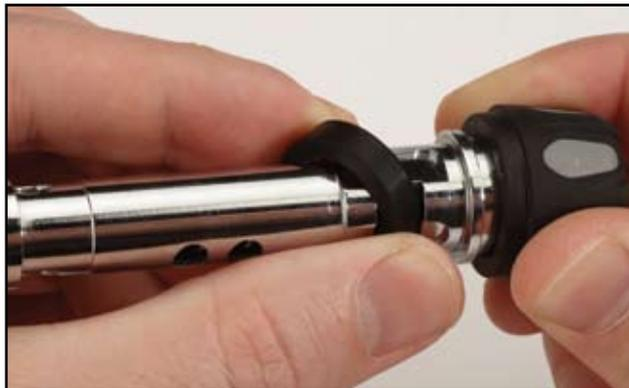
18. Rotate the control Knob **(20)** counterclockwise until the adjuster body subassembly **(17)** separates from the Valve Body **(9)**. Set the assembly aside for later disassembly. The Poppet **(11)**, Spring **(13)** and Balance Chamber **(14)** will release from the Valve Body. Remove and discard O-ring **(12)**. Remove the Seat **(10)** by grasping and pulling lightly. Discard the seat. Set aside the Balance Chamber **(14)**, Poppet **(11)** and Spring **(13)** for cleaning and reassembly.
