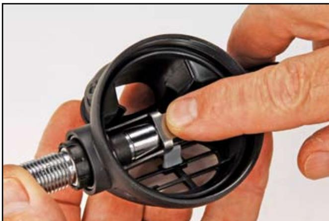
12. It is not generally necessary to remove the Exhaust Valve **(33)** from the Body for cleaning and inspection. However if it is removed, be certain to use the technique that is least stressful to the Exhaust Valve by folding it over and pinching it between the fingers while grasping the tab and gently pulling in opposite directions to elongate the tab as it passes through the rectangular hole in the Housing. Set aside both parts for cleaning, inspection and reassembly.
