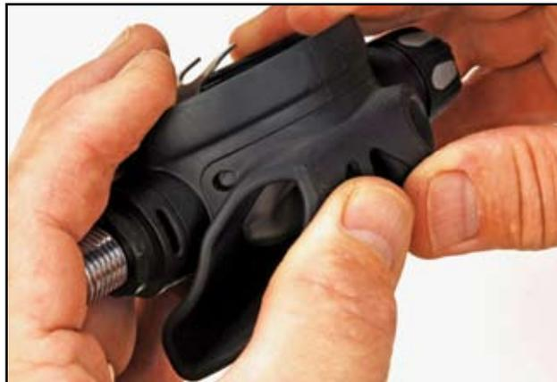
17. Install a lubricated new O-ring (4) in the LP Hose (1) and attach the Hose to the Valve Body. Move the Hose Protector (27) to the fully seated position.
