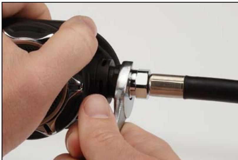
5. Remove the Front Cover Assembly by grasping the Cover Ring (**23**) and rotating it counterclockwise. Inspect the flexible Cover (**24**) for signs of tears, holes or other damage. Replace if damage is evident. If no damage is found go to step 7.
