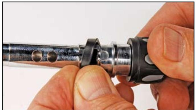
3. Install the Lever Saddle (7) over the Valve Body taking care to align the tab under the threaded area of the Lever Saddle with the slot in the outer surface of the Valve Body.
