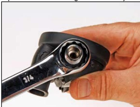
11. While depressing the Lever **(8)** fully with one hand, push on the threaded end of the Valve Body **(9)** to remove the entire subassembly from the Housing **(30)**. O-ring **(29)** will release from the Body. Set it aside for cleaning and reassembly.
