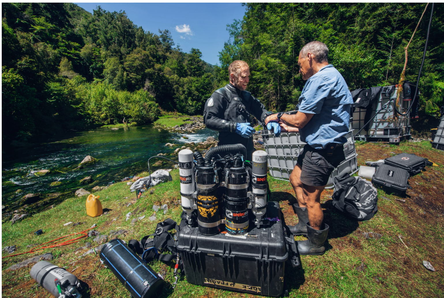
Challen helps Harris gear up in 2020; in front are dual Megalodon rebreathers, one containing an oxygen-helium-hydrogen mix, the other the standard oxygen-helium-nitrogen.
