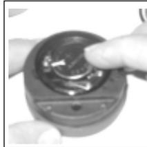
Fig. 49 - Inserting Battery
