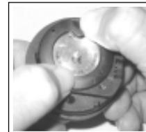
Fig. 52 -Engaging Retaining Ring
