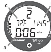
Fig. 4 - Time Displays & Temperature (Surface)
