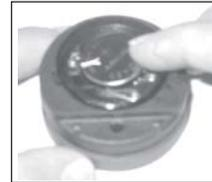
Fig. 92 -Inserting Battery
