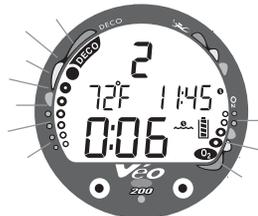
Fig. 60 - Immediate Violation Gauge Mode (after surfacing)
