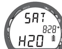
Fig. 77 - Desaturation Mode
