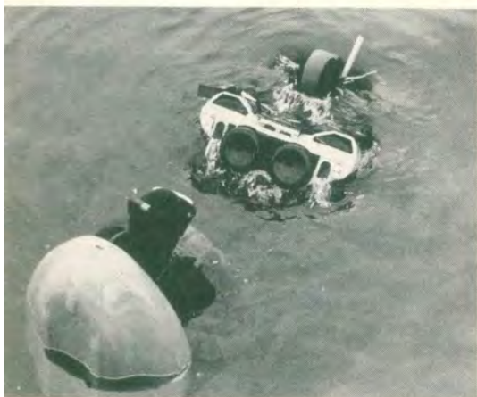
Divers Bernie Campoli and Bill Miller tried the At-Pac in open water. They found it easiest to put the unit on in the water, letting it slip over their heads. Lead shot weights are held in the unit by a trap door, shown below.
