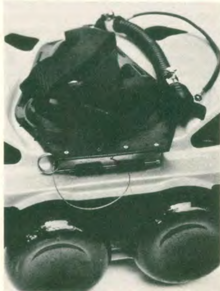
Divers Bernie Campoli and Bill Miller tried the At-Pac in open water. They found it easiest to put the unit on in the water, letting it slip over their heads. Lead shot weights are held in the unit by a trap door, shown below.
